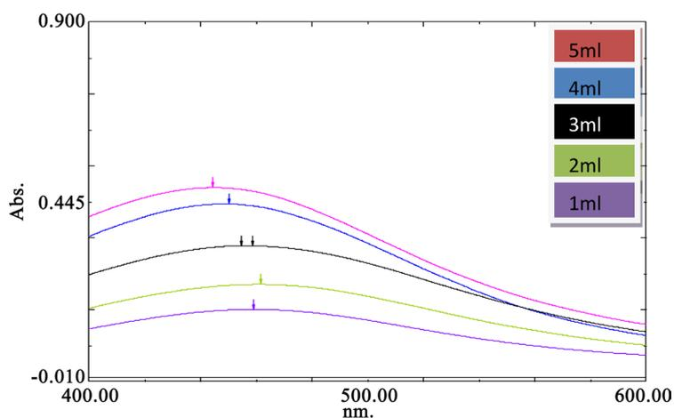
**Figure 2.** UV-visible spectrum of synthesized silver nanoparticles (AgNPs) using different volumes of the extracts (1 - 5 ml).
