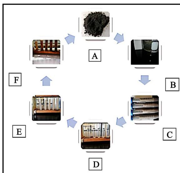
**Figure 1.** Biosynthesis of Silver nanoparticles. (A) Powder of *N. sativa* seeds; (B) homogenized suspension; (C) The extract after centrifugation; (D) Silver nitrate 1 M (10 ml); (E) & (F) The process of reduction after addition of the extract indicated by changing in color.
