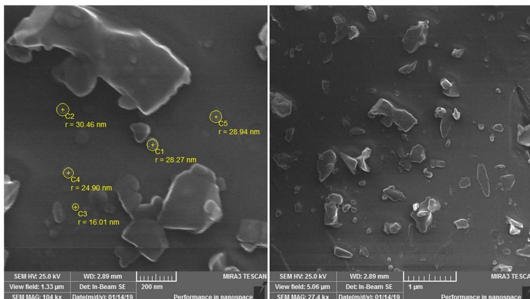
**Figure 3.** SEM analysis of silver nanoparticles synthesized from *Nigella sativa*.
