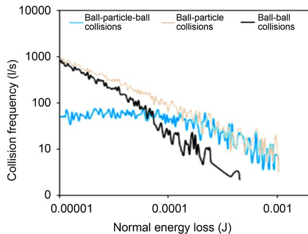
**Figure 3.** Variation of collision frequency with energy loss for different types of collisions.
