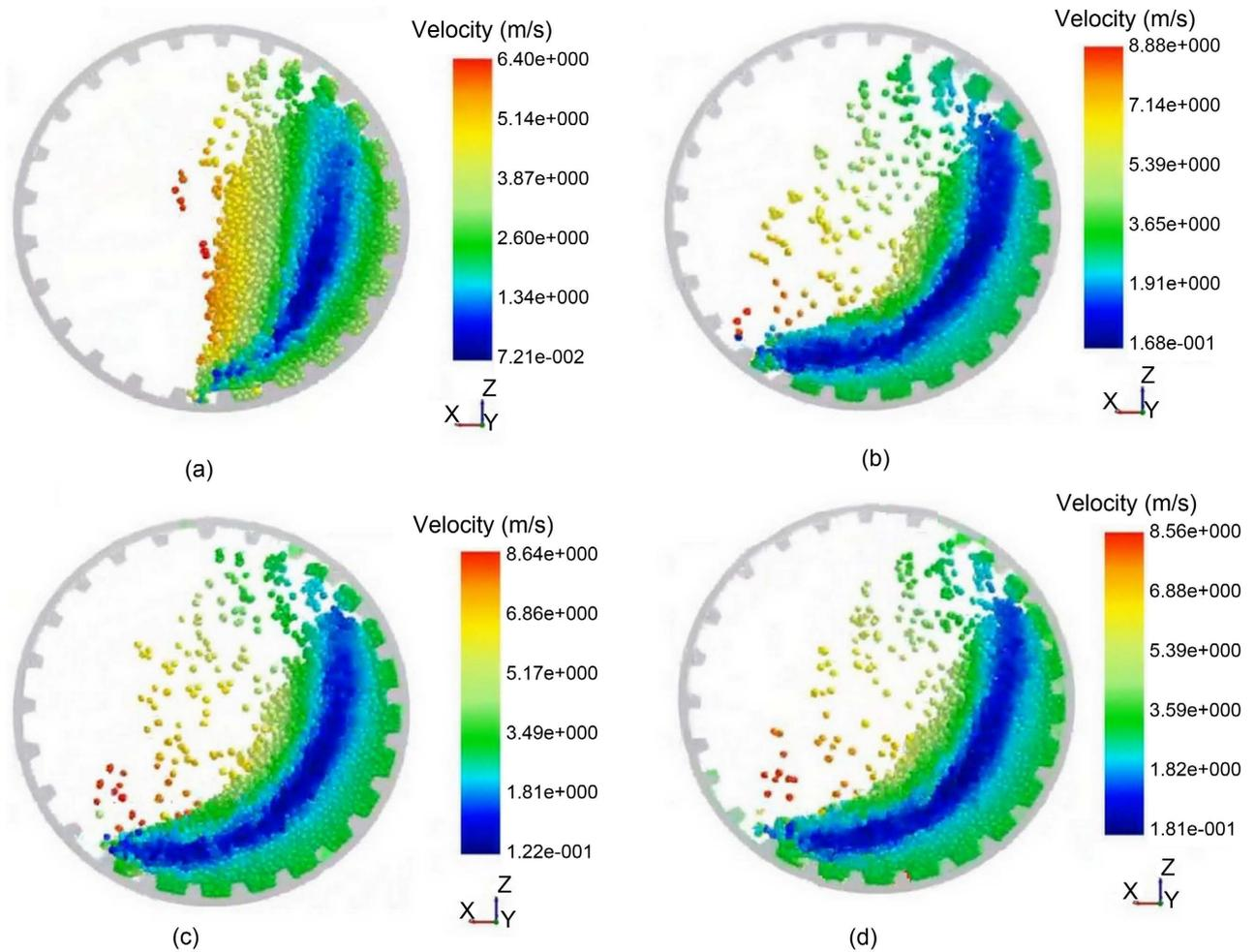
**Figure 2.** Snapshots of particles in planetary mill at different stages of particle breakage.
