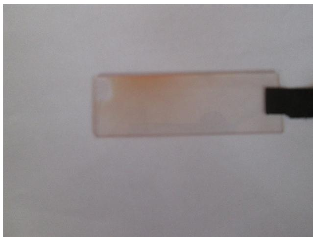
**Figure 5.** The Sudan III thin film result of the PVD method on the glass slide substrate.
