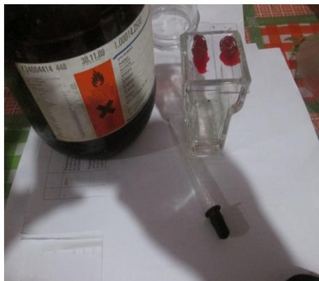
**Figure 3.** The experimental setting of Sudan III thin film exposed to acetone vapor or alcohol vapor.
