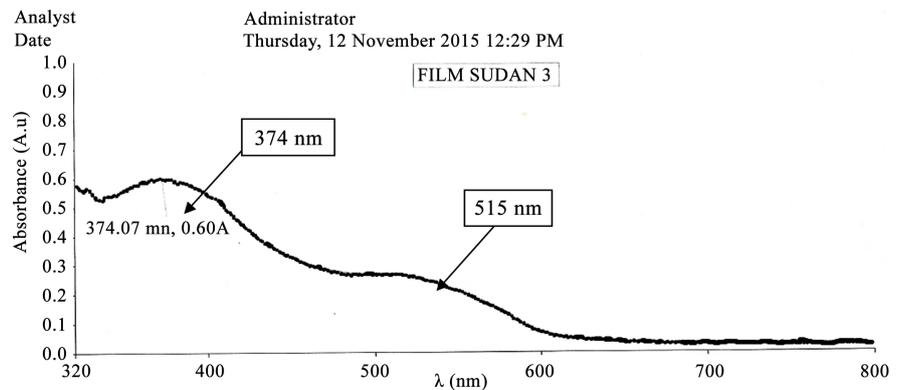
**Figure 10.** UV-VIS spectra of Sudan III thin film results of vacuum evaporation deposition.
