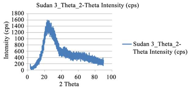
**Figure 8.** The XRD spectra of Sudan III film exposed to alcohol vapor.
