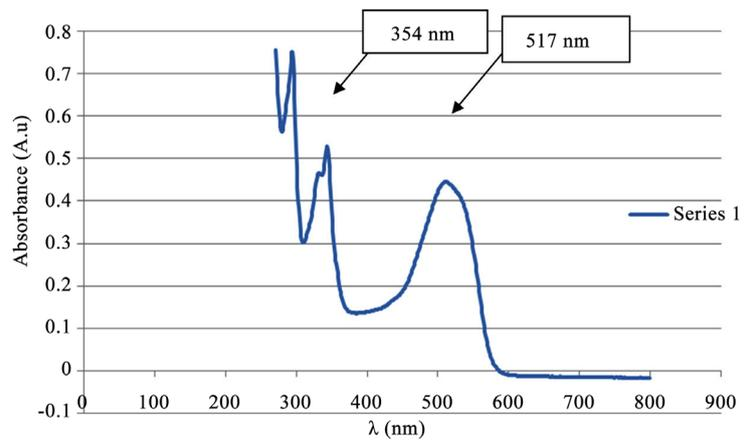
**Figure 9.** UV-VIS spectra of Sudan III solution (Chloroform Solvent).
