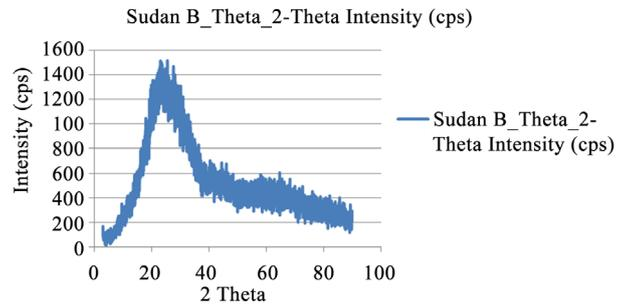
**Figure 7.** The XRD spectra of Sudan III thin film exposed to acetone vapor.
