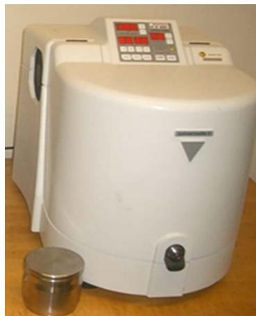
**Figure 1.** Photograph of the high-energy planetary ball mill.
