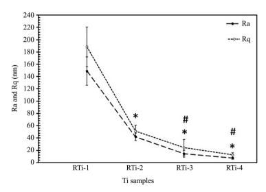
**Figure 2.** Uncoated Ti samples displayed a gradual decrease in average roughness (Ra) and root mean square roughness (Rq) as a result of mechanical polishing. n = 5; \* p < 0.05 compared to RTi-1; # p < 0.05 compared to RTi-2.
