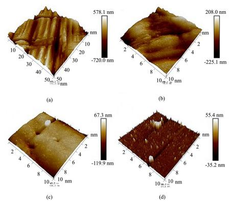
**Figure 1.** AFM images of uncoated Ti surfaces with four degrees of roughness; (a) RTi-1; (b) RTi-2; (c) RTi-3; (d) RTi-4.
