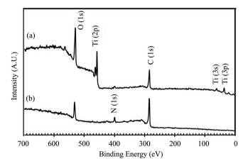
**Figure 4.** XPS spectra from the surface of (a) RTi-1 (uncoated Ti) and (b) CRTi-1 (coated Ti with PDA monolayer).
