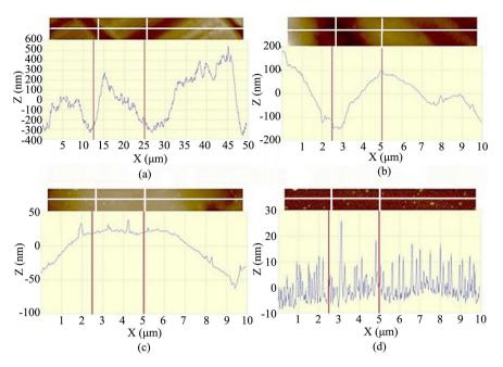
**Figure 3.** Height profile along the white line marked in each AFM image; (a) RTi-1; (b) RTi-2; (c) RTi-3; (d) RTi-4.
