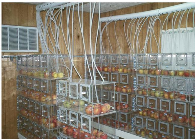
**Figure 1.** Ripening chambers at the University of Idaho Pomology and Viticulture Program laboratories were used to evaluate evolved ethylene and respiration of apples.
