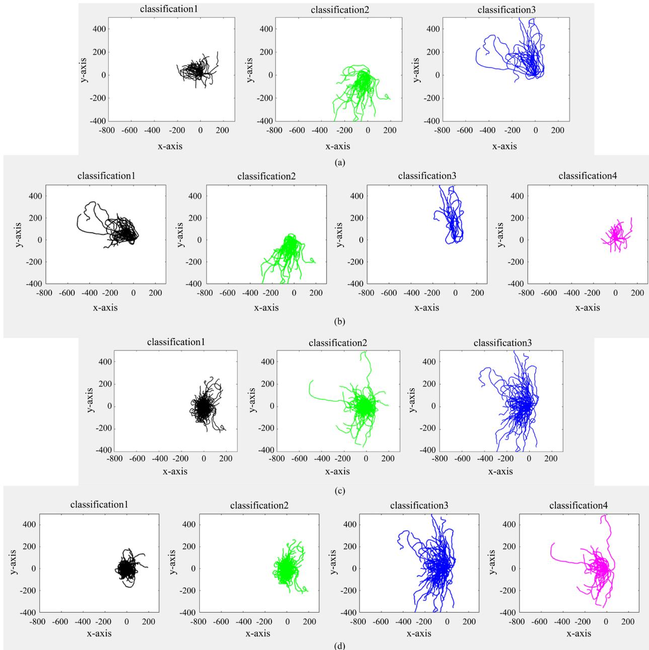
**Figure 5.** Classification results under different normalization methods. (a), (b) Trajectories vectors normalization, one is set as three groups and another is four. (c), (d) Geometric features normalization, and the classification results are similar.
