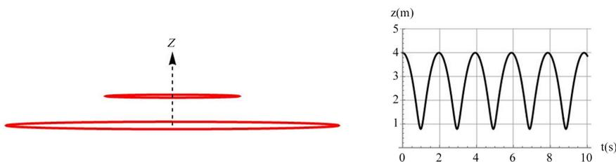
**Figure 6.** Screen shot of the simulation of the oscillations of the floating ring. The left panel is the actual oscillator, the right panel is the oscillating position of the ring vs. time.
