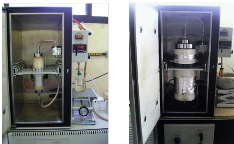
Figure 1. Supercritical fluid equipment with a capacity of 0.1 L and 1.0 L (photo by author).
