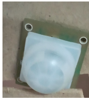
Figure 9. A HC-SR501 PIR sensor attached to the walls of the smart-office system.
