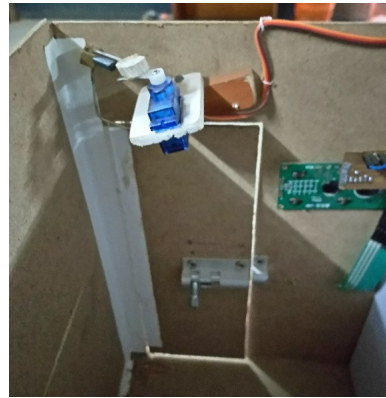
Figure 6. TowerPro SG90 Servo Motor that opens the outer door.
