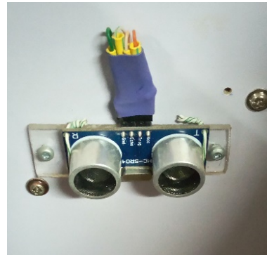
Figure 7. An ultra-sonic sensor HC-SR04 attached in the corridor.
