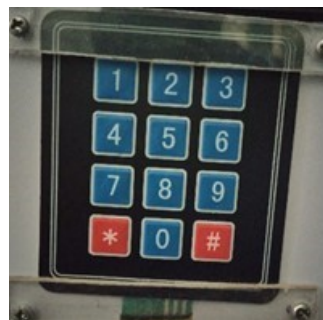
Figure 5. A 4 \times 3 keypad for the outer door.
