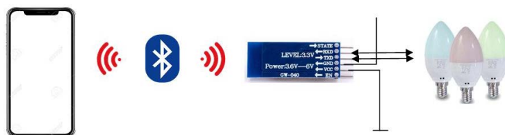
Figure 13. Illustrates how an Android phone is connected to Bluetooth and the 3 LED bulbs.
