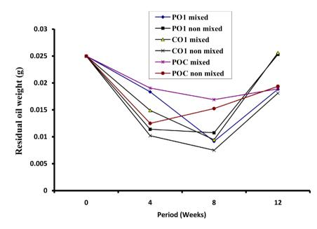
Figure 9. Total recoverable residual oil in sterile oil mill sample with and without mixing.
