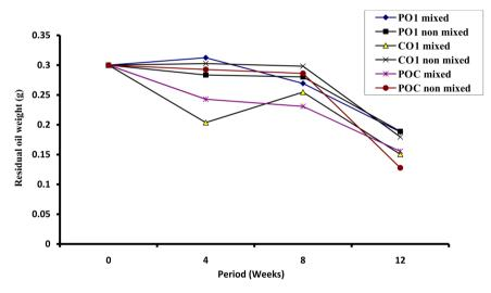
**Figure 13.** Total recoverable residual oil in sterile palm kernel oil contaminated sample with and without mixing.
