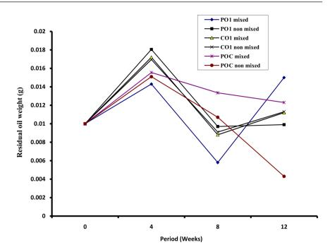
Figure 10. Total recoverable residual oil in non-sterile oil mill sample with and without mixing.
