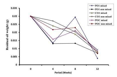
Figure 12. Total recoverable residual oil in non sterile unpolluted sample with and with out mixing.
