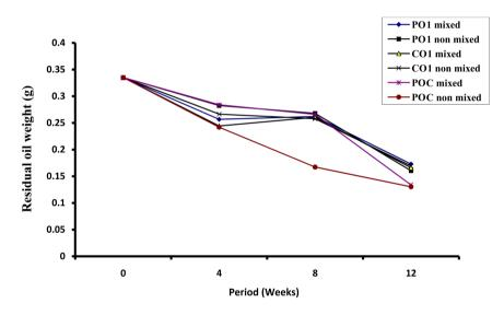
**Figure 15.** Total recoverable residual oil in sterile palm oil contaminated sample with and without mixing.
