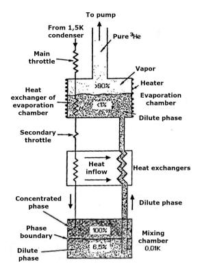
**Figure 1.** Typical diagram of the <sup>3</sup>He/<sup>4</sup>He refrigerator.
