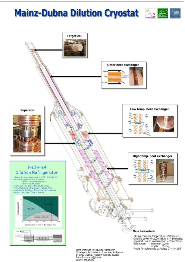
Figure 11. Main units and parameters of the polarized target cryostat in Mainz.
