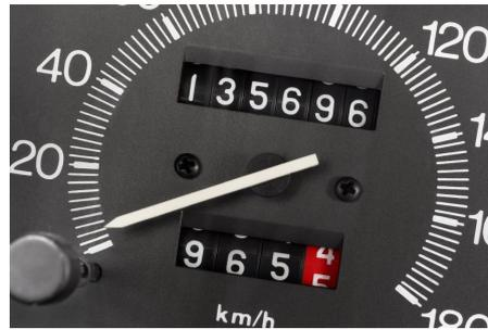
**Figure 1.** An odometer and a trip meter installed in a modern car.
