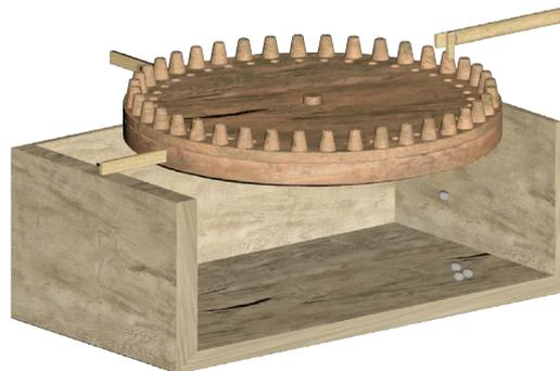
**Figure 10.** Peg wheel and drum with pebbles.
