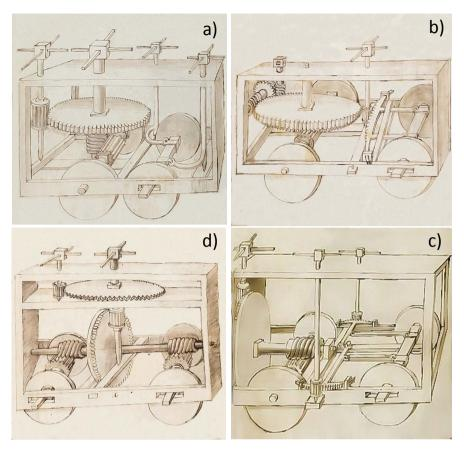
**Figure 4.** Designs of four-wheel vehicles set in motion by manually driven gears and with directional control. Francesco di Giorgio. *Opusculum de Architectura*, (a) folio 3r, (b) folio 29v, (c) folio 31r e (d) folio 4r (details). British Library Museum. London. UK.
