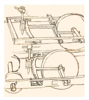
**Figure 2.** Study of a steering system to control the direction of the vehicle movement. Francesco di Giorgio. *Codicetto Vaticano*, folio 115r (detail). Biblioteca Apostolica Vaticana. Rome. Italy.
