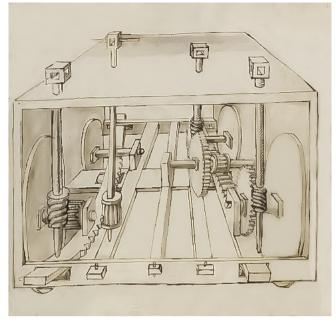
**Figure 8.** 3D drawing of a self-propelled vehicle. Francesco di Giorgio. *Opusculum de Architectura*, folio 26v (detail). British Library Museum. London. UK.
