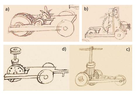
**Figure 1.** Three-wheeled vehicle designs set in motion through manually operated gears. Francesco di Giorgio. *Codicetto Vaticano*, (a) e (b) folio 76v, (c) folio 107r e (d) folio 107v (details). Biblioteca Apostolica Vaticana. Rome, Italy.
