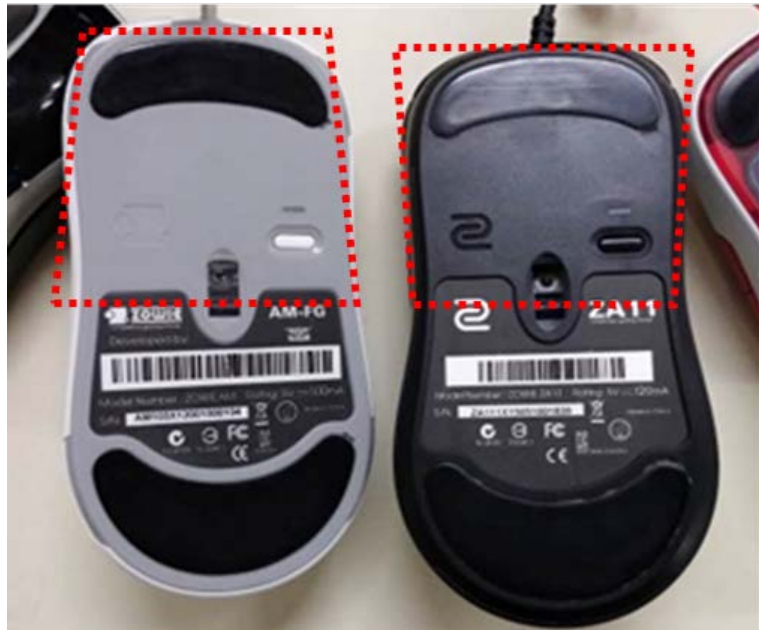
Figure 11. Up-trapezoidal mouse (left) has a wider middle part and milder concave and is less likely to be held tightly, while the up-trapezoidal mouse (right) has a greater concave in the middle and is more likely to be held tightly.
