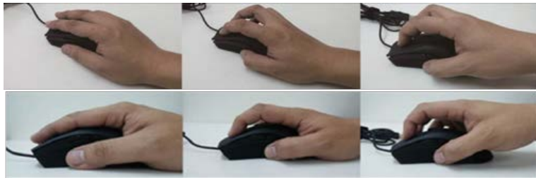
Figure 4. Three basic mouse postures for players (left to right): bend-over holding, grasp holding, and click holding.
