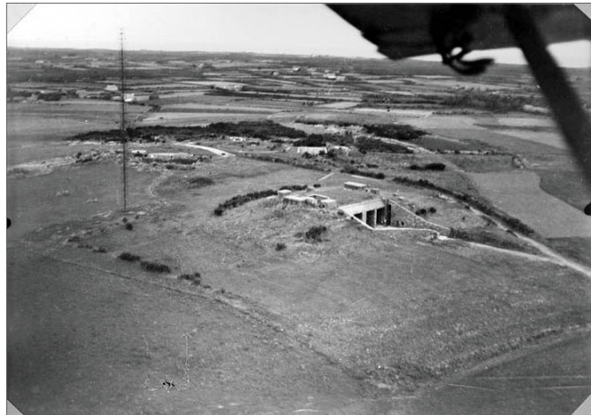
Figure 1. aerial oblique view of the radio guidance station K11, Stp Mo 44c of Saint-Fiacre around 1947. Distinguishable are: the access road, the reinforced, buried bunker, concrete barracks or exhaust vents near the bunker, Flak emplacements, the Knickebein ring with two nearby constructions, a ditch for one shack or cistern; the Wasserman/See Elefant antenna (Rapport Pinczon du Sel, 1947-1948a).
