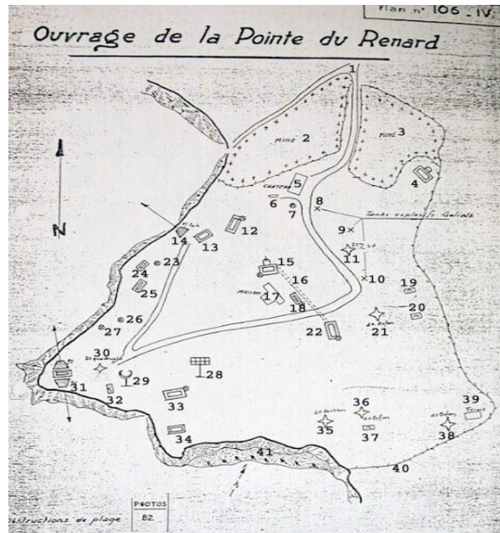
Figure 1. Stp Kerlohic (Re 57-58 ; Re120-123), Pointe du Renard (Le Conquet)-map from: Plan n° 106_IV ( Rapport Pinczon du Sel, 1947-1948 ): (1) access road; (2) - (3) minefield; (4) unburied concrete bunker surmounted by an armoured cupola for machine gun and grenade launcher; (5) castle-headquarter residence; (6) castle dependence; (7) tobruck for machine gun; (8) - (10) explosive tank Goliath garages; (11) concrete platform for Flak gun-small model-25 mm S-A; (12) unburied thick concrete bunker flanked by a tobruck for machine gun; (13) unburied concrete bunker or hold; (14) concrete bunker for anti-tank gun-37 PaK ; (15) unburied thick concrete bunker flanked by a tobruck for machine gun surmounted by an armored cupola for periscope; (16) concrete tunnel; (17) house-soldier lodgement; (18) unburied concrete bunker or hold; (19)-(20) lightweight concrete bunker or hold; (21) concrete platform for Flak gun-small model-40 Bofors; (22) unburied thick concrete bunker flanked by a tobruck for machine gun; (23) tobruck for machine gun; (24) - (25) unburied concrete bunker or hold; (26) - (27) tobruck for machine gun; (28) large format marine search radar; (29) anti-aircraft search radar; (30) concrete platform for Flak gun-small model-20 quadruple; (31) double concrete bunker for anti-tank gun; (32) lightweight concrete bunker or hold; (33) buried thick concrete bunker flanked by a tobruck for machine gun; (34) unburied concrete bunker or hold; (35) concrete platform for Flak gun-small model-20 Oerlikon; (36) concrete platform for Flak gun-small model-40 Bofors; (37) lightweight concrete bunker or hold; (38) concrete platform for D.C.A gun-small model-40 Bofors; (39) farm; (40) barbed wire; (41) tetrahedral pyramids and wooden piles-beach obstacles.
