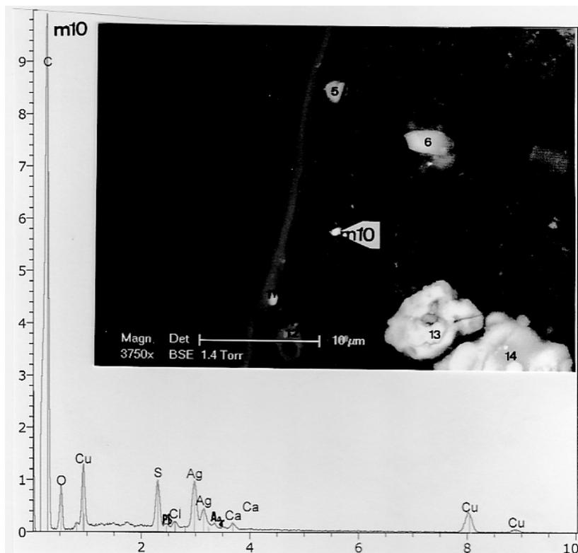
**Figure 19.** The m10 particle. *Above:* SEM photograph (3750×), in BSE, of the m10 particle (m5 and m6: montmorillonite particles; m11: a calcite particle). *Below:* the spectrum of m10. C: carbon; O: oxygen; Cu (three peaks): copper; S: sulphur; Pb (traces): lead; Ag (three peaks): silver; Ca (two peaks): calcium.
