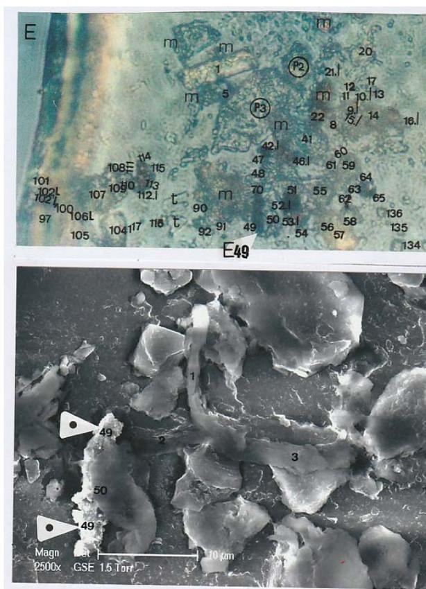
**Figure 1.** The e49 particle. *Above:* optical view ( $500\times$ ) of the E area, showing the e49 particle. *Below:* SEM photograph ( $2500\times$ ), in GSE, of e49; the two apparent parts (superior and inferior), designed as pointed triangles, of e49 are partially separated by the left superior part of e50 (a Cyanophyceae). 1, 2 and 3 indicate the three different parts of FL.4 (linen fiber number 4).
