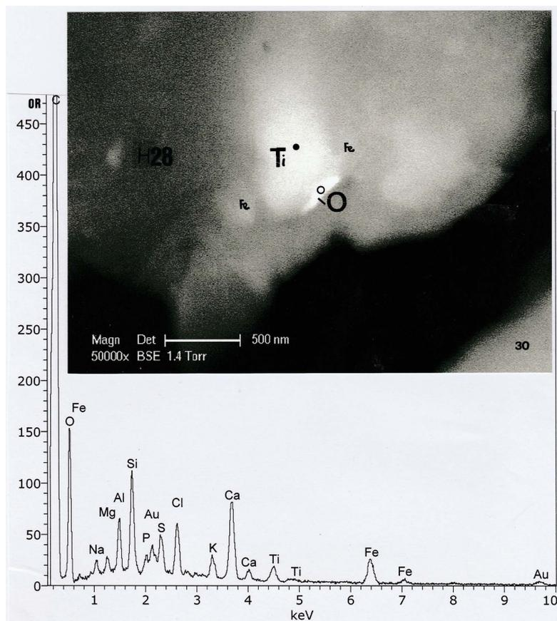
**Figure 13.** Above: SEM photograph (50,000 $\times$ ), in BSE, of the lower part of the h28 particle (30: some part of the h30 particle). Ti: titanium sub-particle; Fe: iron sub-particles; o: gold sub-particle. Below: spectrum of the o sub-particle. C: carbon; O: oxygen; Fe (three peaks): iron; Na: sodium; Mg: magnesium; Al: aluminium; Si: silicium; P: phosphorous; Au (two peaks): gold; S: sulphur; Cl: chlorine; K: potassium; Ca (two peaks): calcium; Ti (two peaks): titanium.
