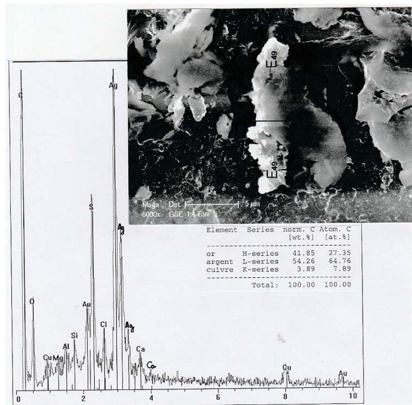
**Figure 2.** Above: SEM photograph (6000×), in GSE, showing the two parts of the e49 particle. Below: spectrum of e49, in the squared area of the photograph. C: carbon; O: oxygen; Cu (two peaks): copper; Mg: magnesium; Al: aluminium; Si: silicium; Au (two peaks): gold; S: sulphur; Cl: chlorine; Ag (three peaks): silver; Ca (two peaks): calcium. *Insert:* normal composition: or (gold); argent (silver); cuivre (copper).
