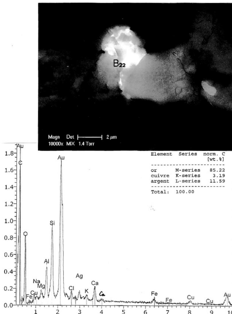
**Figure 5.** Above: SEM photograph (10,000 $\times$ ), in GSE + BSE, of the b22particle. Below: spectrum of b22. C: carbon; O: oxygen; Fe (two peaks): iron; Cu (three peaks): copper; Na: sodium; Mg: magnesium; Al: aluminium; Si: silicium; Au (two peaks): gold; Cl: chlorine; Ag: silver; K: potassium; Ca (two peaks): calcium. *Insert:* normal composition: or (gold); cuivre (copper); argent (silver).
