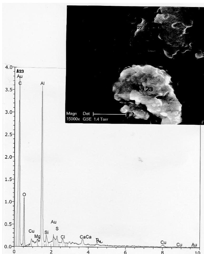
**Figure 10.** Above: SEM photograph (15,000 $\times$ ), in GSE, of the a23 particle (a22 and a22' are other similar particles). Below: spectrum of a23. C: carbon; Au (three peaks): gold; O: oxygen; Cu (three peaks): copper; Mg: magnesium; Al: aluminium; Si: silicium; S: sulphur; Cl: chlorine; Ca (two peaks): calcium; Ba: barium.
