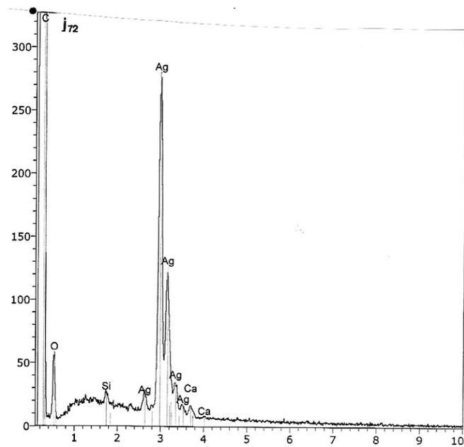
**Figure 15.** The j72 spectrum (in a dot). C: calcium; O: oxygen; Si: silicium; Ag (five peaks): silver; Ca (two peaks): calcium.
