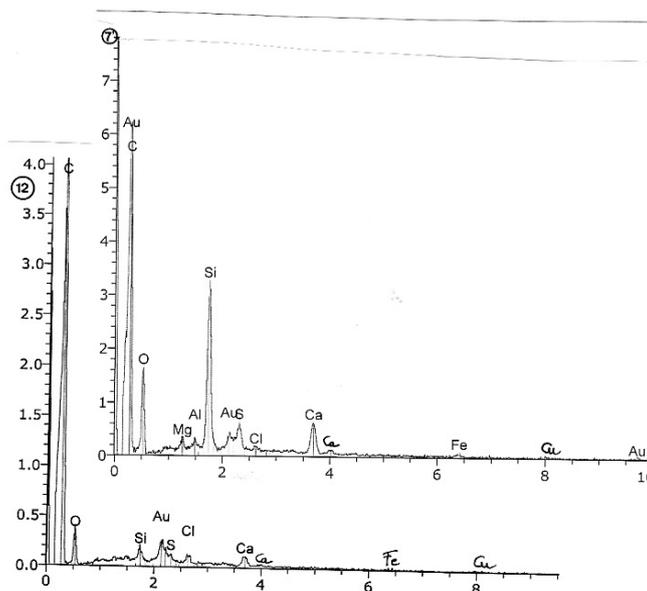
**Figure 9.** Spectras of sub-particles 7' and 12. C: carbon; Au (three peaks): gold; O: oxygen; Mg: magnesium; Al: aluminium; Si: silicium; S: sulphur; Cl: chlorine; Ca (two peaks): calcium; Fe: iron; Cu: copper.
