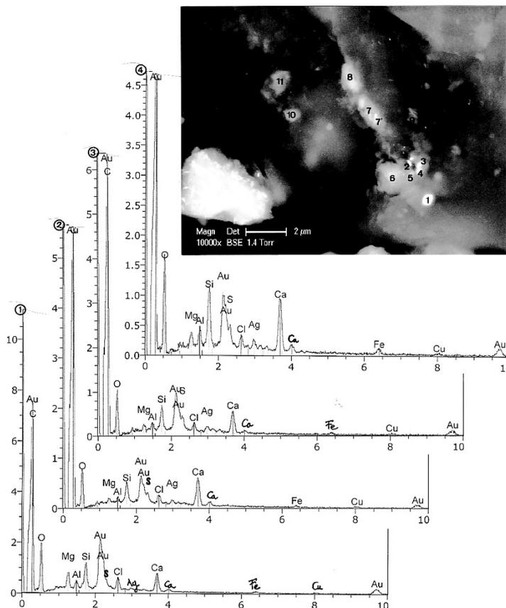
**Figure 8.** Above: SEM photograph (10,000×), in BSE, of the part of the I38 particle showing sub-particles 1, 2, 3, 4, 5, 6, 7, 8, 9, 10 and 11. Below: spectras of sub-particles 1, 2, 3 and 4. C: carbon, O: oxygen; Au (four peaks): gold; Mg: magnesium; Al: aluminium; Si: silicium; S: sulphur; Cl: chlorine; Ag: silver; Ca (two peaks): calcium; Fe: iron; Cu: copper.
