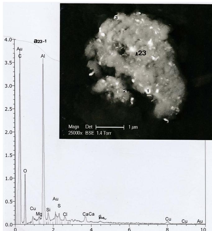
**Figure 11.** Above: SEM photograph (25,000 $\times$ ), in BSE, of the a23 particle; 1, 2 and 3: sub-particles on a23. Below: spectrum of sub-particle 1. C: carbon; Au (three peaks): gold; O: oxygen; Cu (three peaks): copper; Mg: magnesium; Al: aluminium; Si: silicium; S: sulphur; Cl: chlorine; Ca (two peaks): calcium; Ba: barium.
