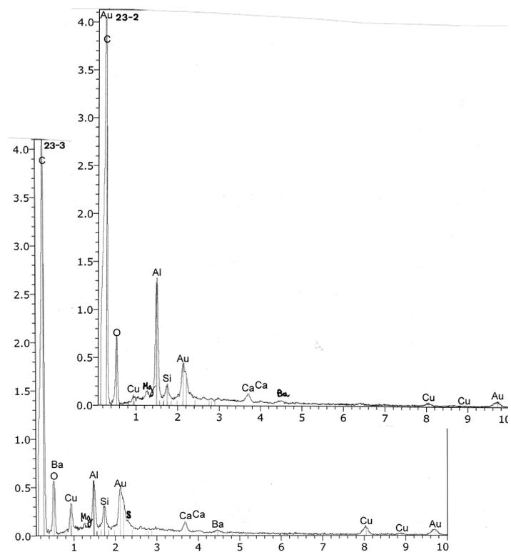
**Figure 12.** Spectras of sub-particles 2 and 3.
