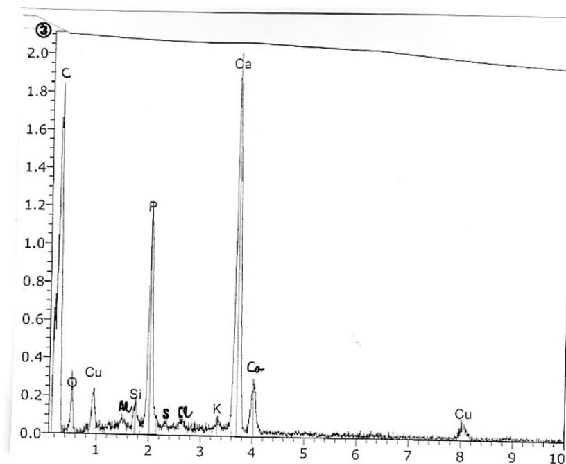
**Figure 20.** Spectrum of sub-particle 3, loaded on particle f13 - f14. C: carbon; O: oxygen; Cu (two peaks): copper; Al: aluminium; Si: silicium; P: phosphorous; S: sulphur; K: potassium; Ca (two peaks): calcium.
