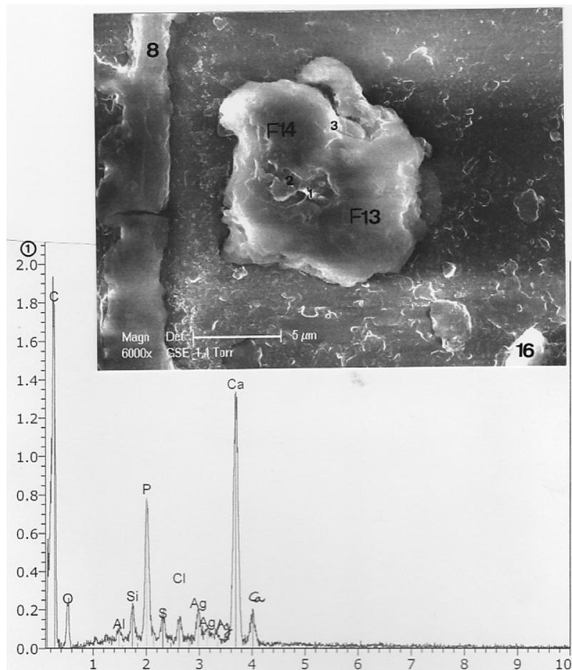
**Figure 17.** The f13 - f14 particle. *Above:* SEM photograph (6000×), in GSE, of the f13-f14 particle (f8: a Diatoms; f16: an hematite; 1, 2 and 3: sub-particles loaded on the f13-f14 surface). *Below:* spectrum of the sub-particle 1. C: carbon; O: oxygen; Al: aluminium; Si: silicium; P (a great peak): phosphorous; S: sulphur; Cl: chlorine; Ag (three peaks): silver; Ca (two peaks): calcium.
