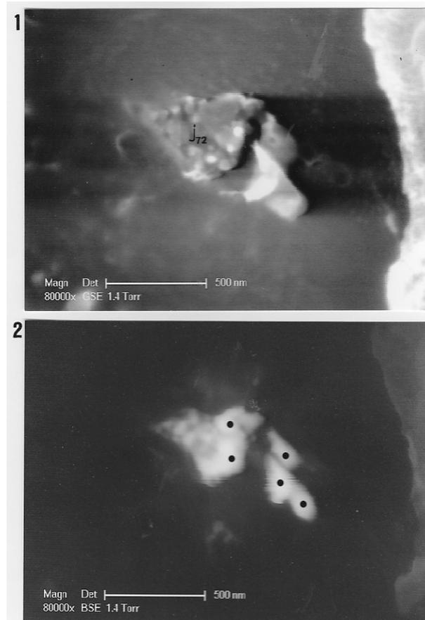
**Figure 14.** The j72 particle. *Above* (1): SEM photograph (80,000×), in GSE, of j72. *Below* (2): SEM photograph (80,000×), in BSE, of j72. (the five black dots indicate the granules where EDX analyses are realized).
