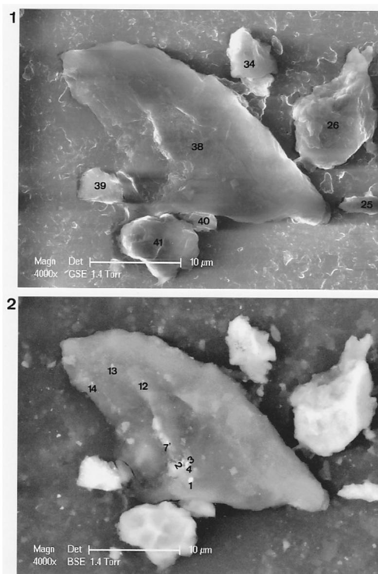
**Figure 7.** Sub-particles of a golden alloy loaded on the l38 particle. *Above (1):* SEM photograph (4000×), in GSE, of the l38 (located in the L area) and other adjacent particles: l26 (a feldspar), l34 (a calcium phosphate); l39 (an hematite); l40 (a silice) and l41 (a quartz). *Below (2):* SEM photograph (4000×), in BSE, of the l38 particle, showing the sub-particles 1, 2, 3, 4, 7, 12, 13 and 14.
