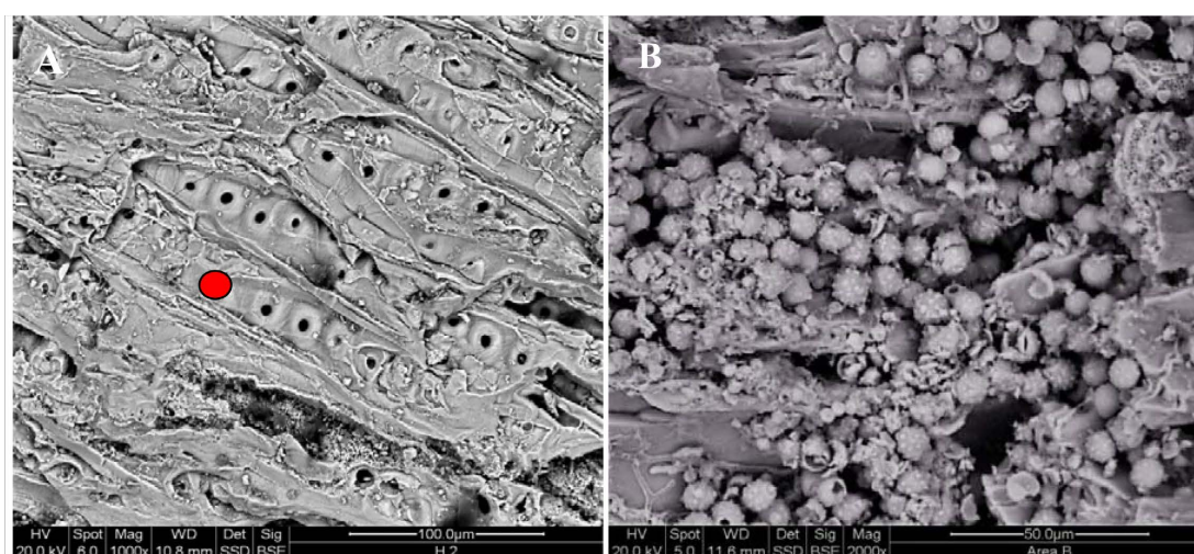
Figure 23. (A) Segment of wood accreted on Nail 2. Tracheids (wood cells with resin channel) show numerous pits in what is probably a tangential section of the cells. The small amounts of Si, Ca and Cl in the wood analyses is caused by contamination from incursions of tunnel moisture, the ~4% carbon concentration is probably all that remains from the original organic carbon. The high Fe content is due to slow replacement of wood carbon by goethite thereby recording one of a number of climate phases which affected the chemistry of the tunnel (see Table 5 , An. 1-7). (B) Wood segment on Nail 1. The organic spheres that colonized the wood are probably spores of the fungus Lycoperdon (Puffball). Individual spheres are 6 - 7 \mu\text{m} in size and exhibit projecting nano-globules ~ 0.5 \mu\text{m} in size.
