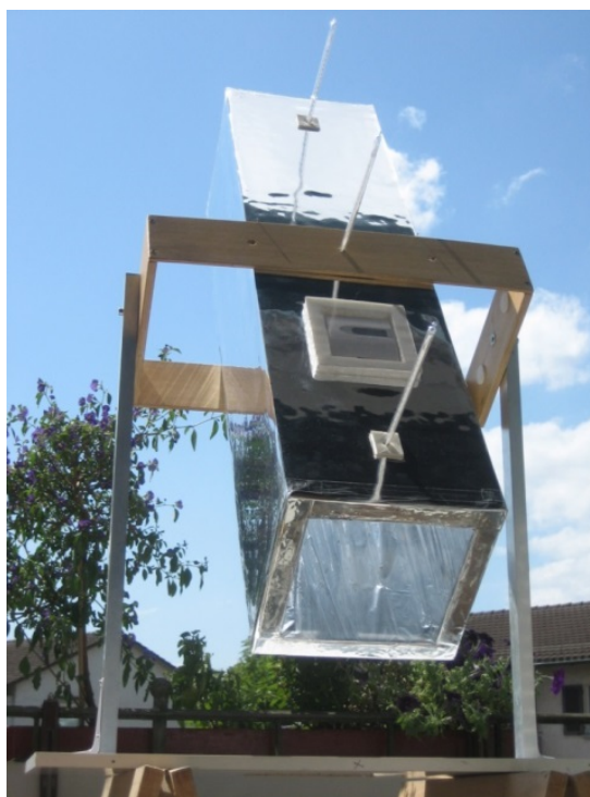
Figure 13. Solar-tube, adjustable to the sun [21].
