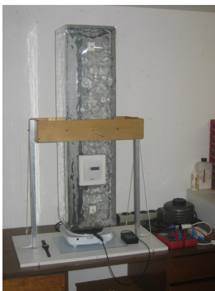
Figure 16. Heat radiation tube with a hot-plate [15].
