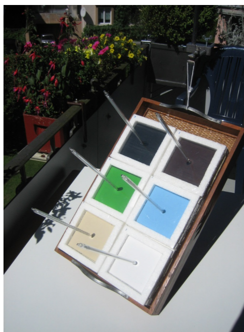
Figure 6. Panel comprising six modules containing different-coloured plates [20].
