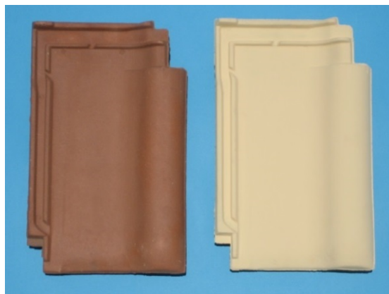
Figure 20. Red-brick original with \beta_s = 0.53 (left) and coloured with \beta_s = 0.30 (right).
