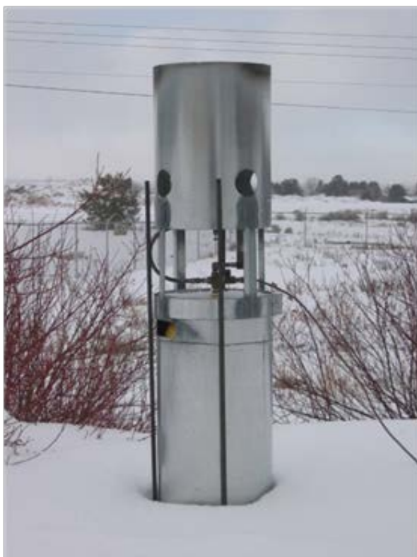
Figure 1. Ground based manually operated Silver Iodide Generator. Courtesy: Griffith et al. [24] (Silver Iodide Generator).
