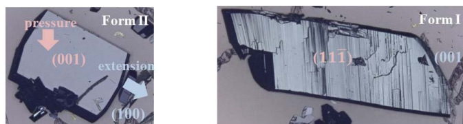
Figure 1. The direction of structural change of Form II before transition and Form I after transition by pressure on Form II crystal surface (001).
