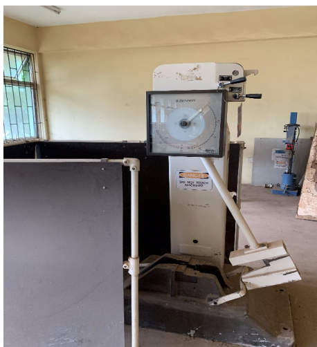
Figure 2. Danison universal pendulum impact system for Izod-Charpy tension and puncture.
