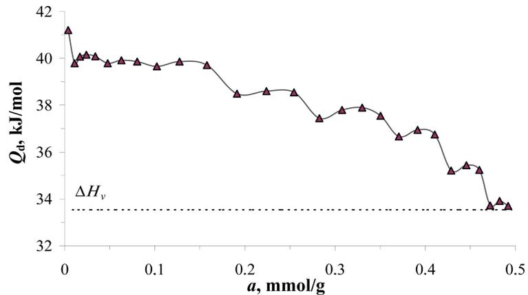
**Figure 2.** Chitosan/Na-CMC at 303 K Differential heat of toluene adsorption on the film membrane: horizontal bar—heat of condensation of toluene.
