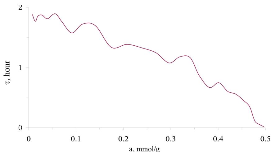
**Figure 4.** Chitosan/Na-CMC at 303 K are the equilibrium time of adsorption of the toluene molecule on the membrane film.
