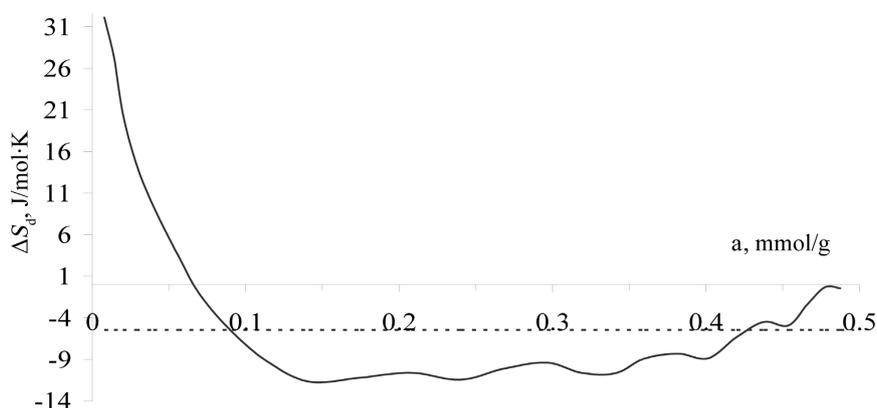
**Figure 3.** Entropy of adsorption of toluene molecule on the membrane of Chitosan/Na-CMC at 303 K: horizontal bar line—average molar integral entropy; the entropy of liquid toluene was assumed to be zero.
