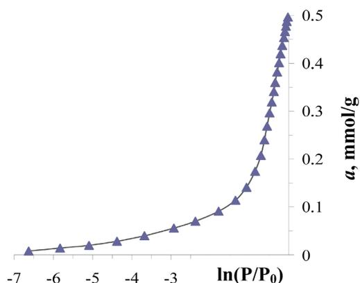
**Figure 1.** Chitosan/Na-CMC toluene adsorption isotherm at film membrane at 303 K.
