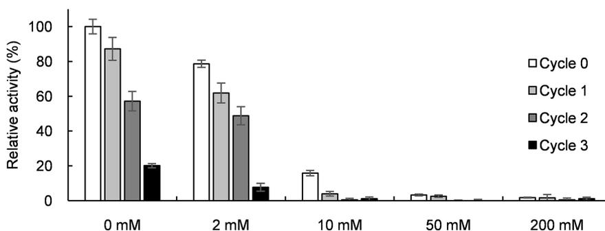
**Figure 4.** Effect of CaCl<sub>2</sub> concentration on the stability of immobilized cells. Immobilized cells (*E. coli*-W525D) were washed for 1 h with 100 mM imidazole buffer (pH 7.5) containing CaCl<sub>2</sub> at concentrations ranging from 0 to 200 mM. After the treatment, enzyme activity present in the wash solution was measured. The values reported for enzyme activity represent the mean  $\pm$  SD (n = 3).
