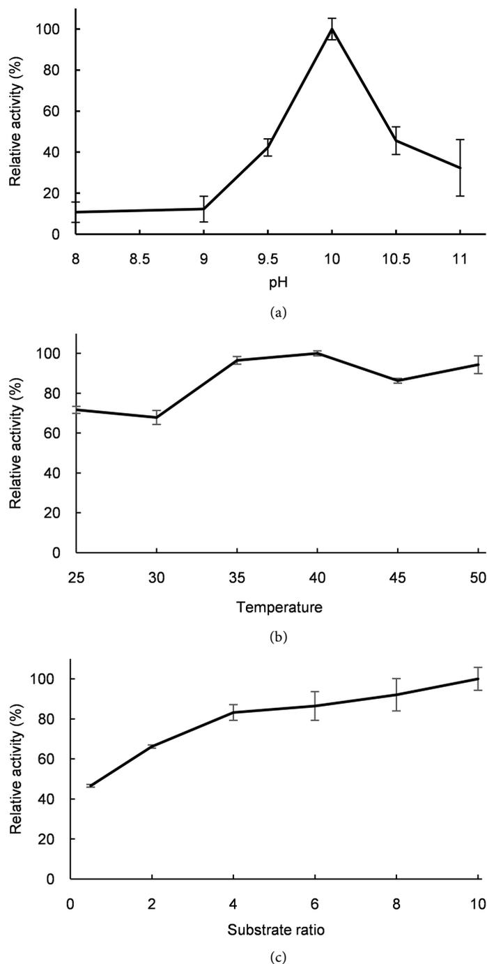
**Figure 1.** L-Theanine production in various conditions with immobilized cells of *E. coli*-W525D mutant. (a) pH-dependence of L-theanine production, pH 8 - 11, (b) Temperature-dependence of L-theanine production, 25°C - 50°C, and (c) Dependence of L-theanine production on the substrate molar ratio using L-Gln and ethylamine and ratios from 0.5 to 10. The values given in the figures represent the mean  $\pm$  SD ( $n = 3$ ).
