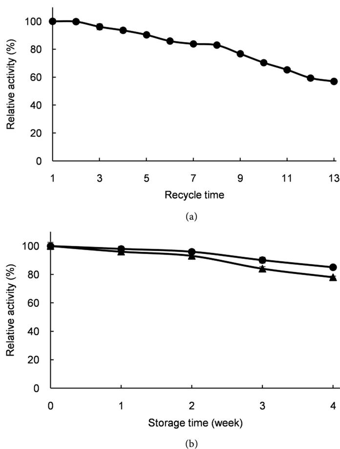
**Figure 5.** Assessment of the reusability and stability of immobilized cells. A) Reusability of immobilized cells; B) Stability of immobilized cells (●) after storage at 4°C and room temperature (▲), The values of activity are hydrolysis activity yields and represent the mean  $\pm$  SD (n = 3).
