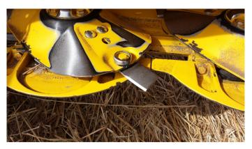
Figure 1. Disc mower blade.
