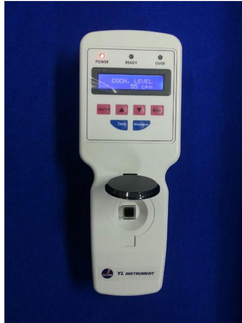
**Figure 6.** Proto-type detector with cuvette for concentration measurement of *Cochlonidium polykrikoides* at 300 nm.
