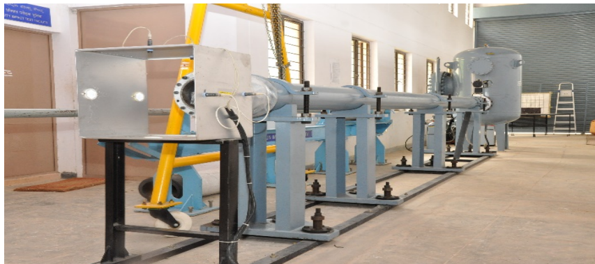
Figure 3. 8/4-lb Bird strike test facility at CSIR-NAL, Bangalore, India.
