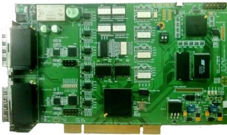
**Figure 3.** Developed DSP-based motion controller.
