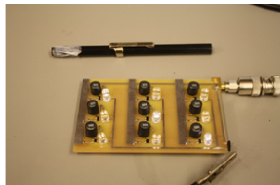
Figure 6. A 3 \times 3 array of controllable LEDs. The pen at the top is used to switch the LEDs by touch.
