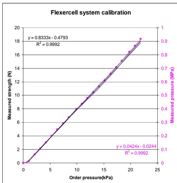
**Figure 1.** Calibration of the compression device using a force sensor.
