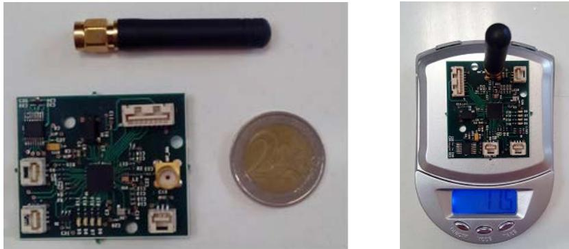
**Figure 1.** Size (a little larger than a 2 € coin) on the left and weight (less than 12 g) of the latest version of RFID tags on the right, without the equipment to recharge it and without battery.
