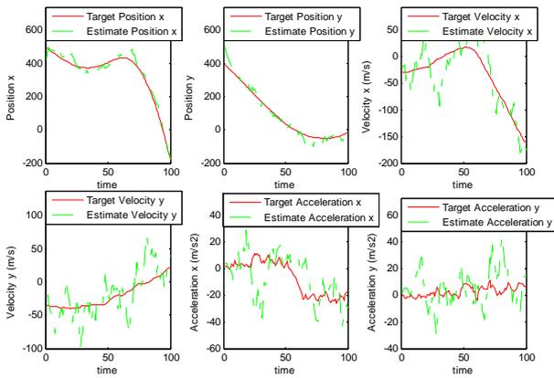
**Figure 7. The estimations of acceleration, velocity, and position along x and y coordinates.**
