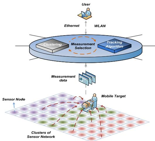
**Figure 1.** The proposed architecture in clusters of sensor network.
