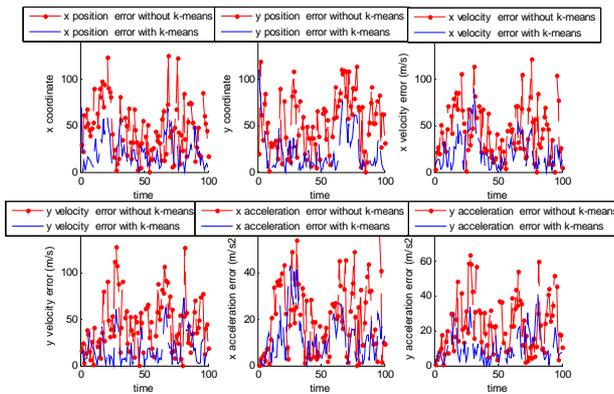
**Figure 9. Comparing the RMSE values for the estimation errors of position, velocity, and acceleration with and without the augmentation of K-means clustering algorithm.**
