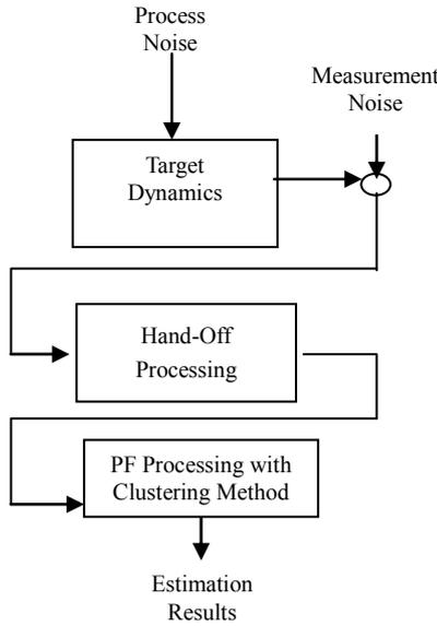
**Figure 2. The block diagram of tracking estimation with clustering analysis.**
