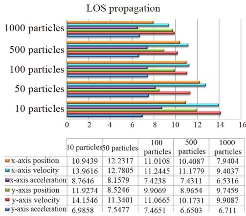
**Figure 12. The results, estimation errors versus numbers of particles, using solely particle filtering in a surrounded LOS propagation environment.**
