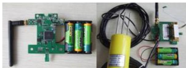
**Figure 1. The NPUnode and equipped sensors.**
