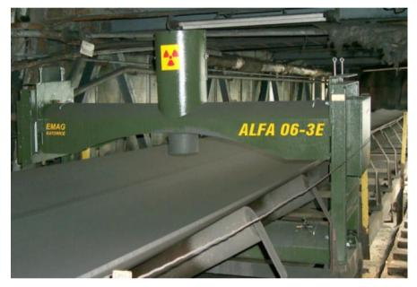
Figure 7. ALFA 06/3E at the coal processing plant Radiation source: 137Cs (0.555 GBq) and 241Am (11.1 GBq) [13].
