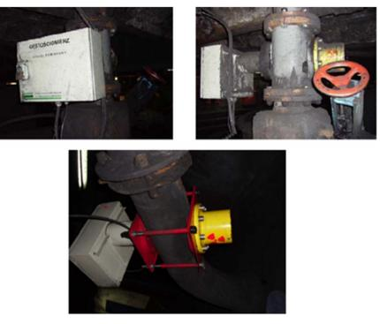
Figure 5. Density gauges into coal enrichment installation (source Cs-137) [13].
