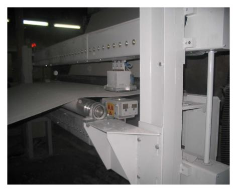
Figure 21. Traversing thickness gauge [25].
