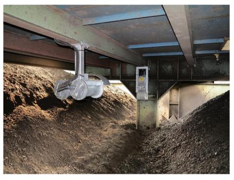
Figure 24. Dust monitoring system in the mine. Detector and radiation emitter (ATEX performance) [26].
