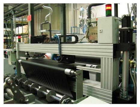
Figure 26. Radiometric profile meter—head with traverse, MM-06 type [26].
