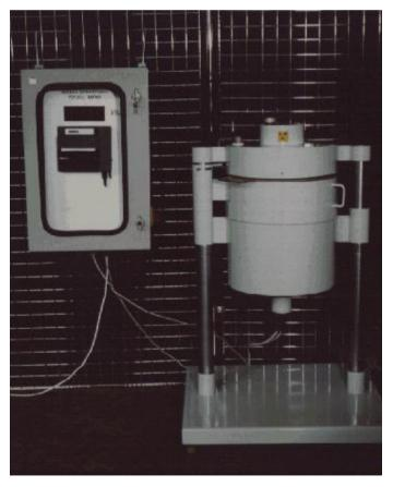
Figure 9. MPKF radiometric ash meter [13].
