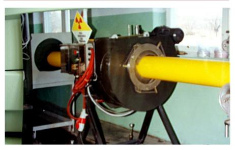
Figure 25. Thickness gauge of plastic pipes walls, MM-04 type [26].
