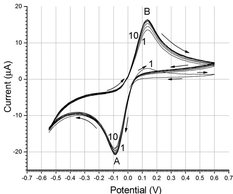
**Figure 3.** Cyclic voltammetry curves of chloranilic acid in presence of uranium drop (around 50 µg/L), pH~3, acidified with H<sub>2</sub>SO<sub>4</sub>, over a SPE electrode (Metrohm E110), using carbon as working electrode and counter-electrode and silver as reference electrode. The numbers at the curves indicate the cycle repetition, where 1 is the first and 10 the last.
