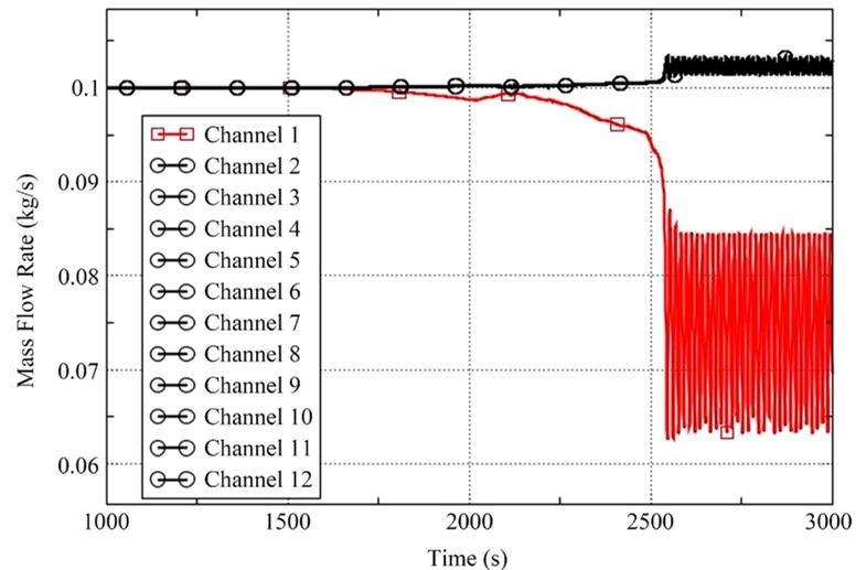
**Figure 18.** RELAP5 calculated mass flow rate for twelve parallel pipes with two fluid model. Stable flow splitting is observed before density waves appear. Eleven channels increase mass flow and the other decrease mass flow.
