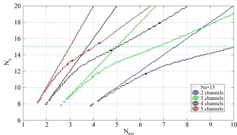
**Figure 10.** Stability map for 2, 3, 4 and 5 identical parallel channels.
