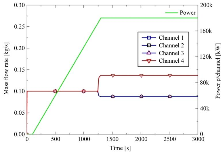
**Figure 15.** RELAP5 calculated mass flow rate for a four parallel pipe arrangement with two fluid model and gravity contribution. The exit concentrated pressure losses coefficient was set to 5. Stable flow splitting is observed.
