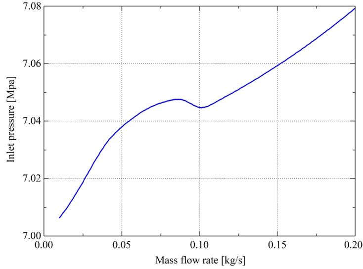
**Figure 1.** Single boiling channel characteristic curve.
