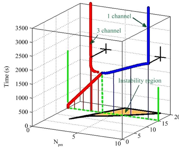
**Figure 16.** RELAP5 calculated  $N_{pM}$  for  $N_s = 15$  in a four parallel pipe arrangement with HEM model and gravity contribution. Representation corresponds to Figure 14. Stable flow splitting is observed.
