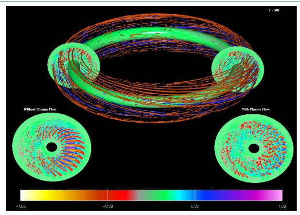
**Figure 4.** Comparison of nonlinear mode structure: effects of zonal flows. GTC simulations, Gyrokinetic Toroidal Code (GTC)<sup>©</sup> Princeton plasma physics laboratory, http://w3.pppl.gov/theory/bin/zonal-flow.jpg
