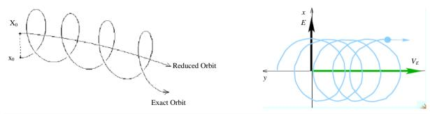
Figure 2. Exact and reduced single-particle orbits in a magnetic field. [5] [7].
