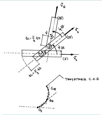
**Figure 6.** The position of the center of mass varies depending on the coupling between the field of the linear velocity and the velocity field caused by the noncoaxial torque [35]. (Figure Alejandro Alvarez).
