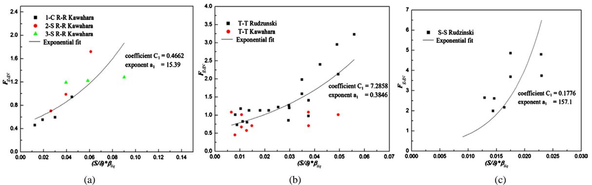
**Figure 9.** The coefficient  $C_1$  and exponent  $a_1$  for various subchannel geometry in gas phase mixing rate.
