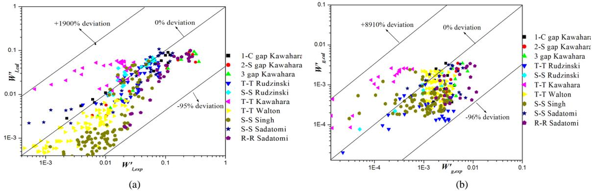
**Figure 4.** Comparison of the predictability of Carlucci *et al.* [11] model against subchannels experiments for liquid and gas phase turbulent mixing rate in two phase flow.
