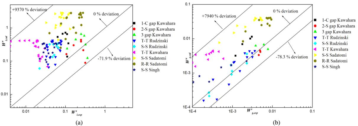
**Figure 3.** Comparison of the predictability of Kawahara *et al.* [10] model against subchannels experiments for liquid and gas phase turbulent mixing rate in two phase flow.
