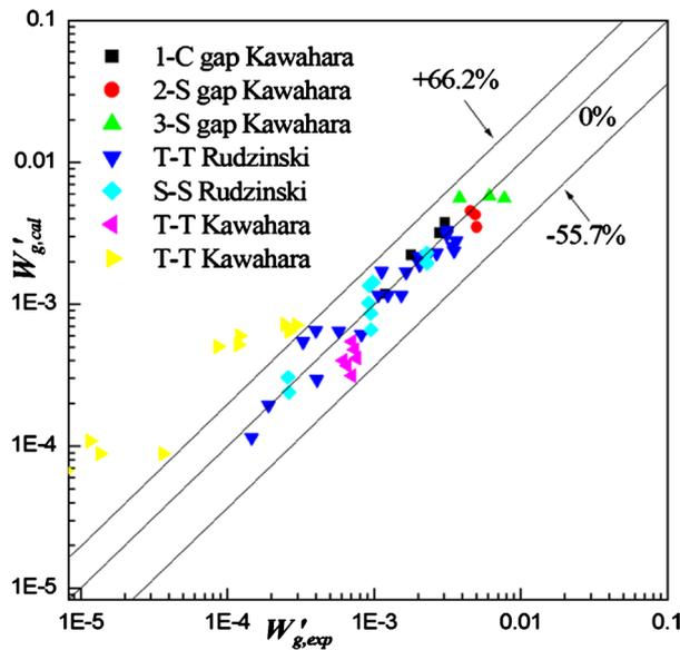
**Figure 11.** Comparison of the predictability of present model against subchannels experiment for Gas phase turbulent mixing rate in two phase flow.
