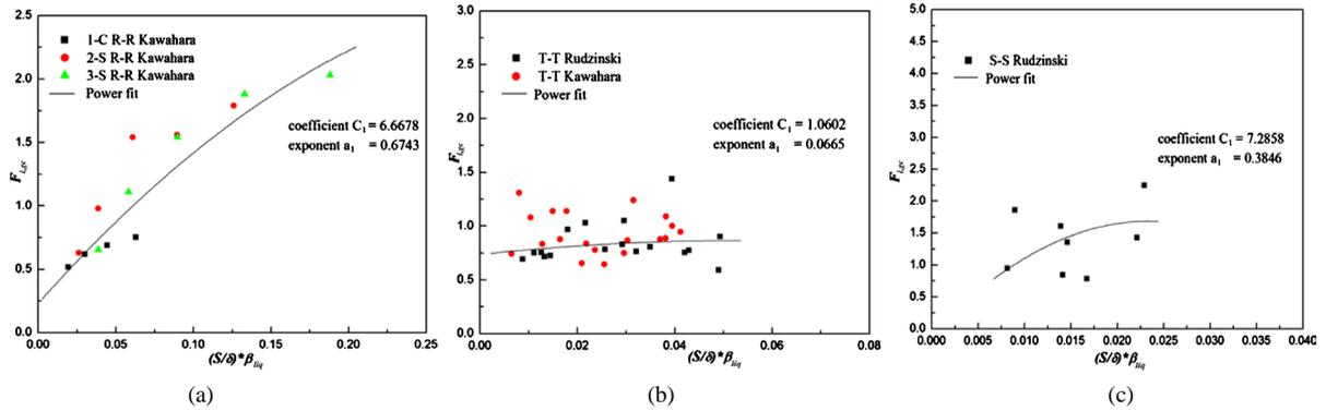
**Figure 8.** The coefficient  $C_1$  and exponent  $a_1$  for various subchannel geometry in liquid phase mixing rate.
