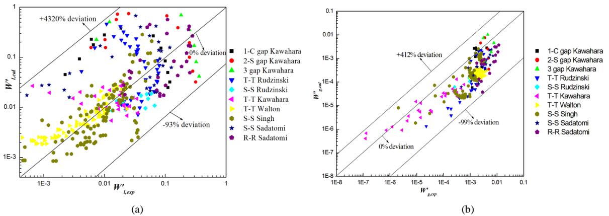
**Figure 1.** Comparison of the predictability of Bues [8] model against subchannels experiments for liquid and gas phase turbulent mixing rate in two phase flow.
