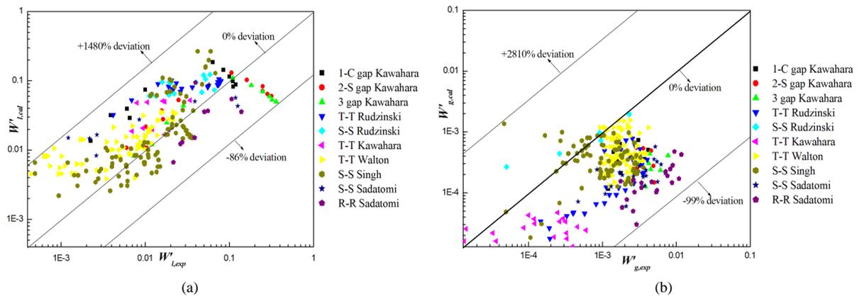
**Figure 2.** Comparison of the predictability of Kazimi and Kelly's [9] model against subchannels experiments for liquid and gas phase turbulent mixing rate in two phase flow.
