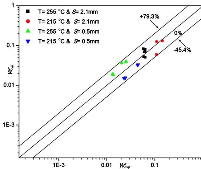
**Figure 12.** Comparison of the predictability of present model against subchannel experiment for total turbulent mixing rate in two phase flow.
