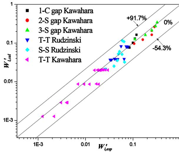
**Figure 10.** Comparison of the predictability of present model against subchannels experiment for liquid phase turbulent mixing rate in two phase flow.
