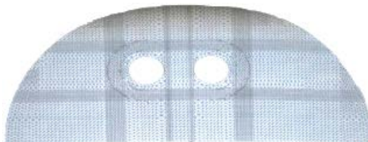
Figure 3. Plan view of the layered shell model showing meshing details.
