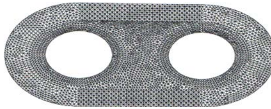
Figure 9. Plan view of mesh type-1 for solid element model.
