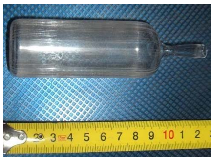
Figure 5. Quartz glass containers are used to irradiate of large crude oil samples.
