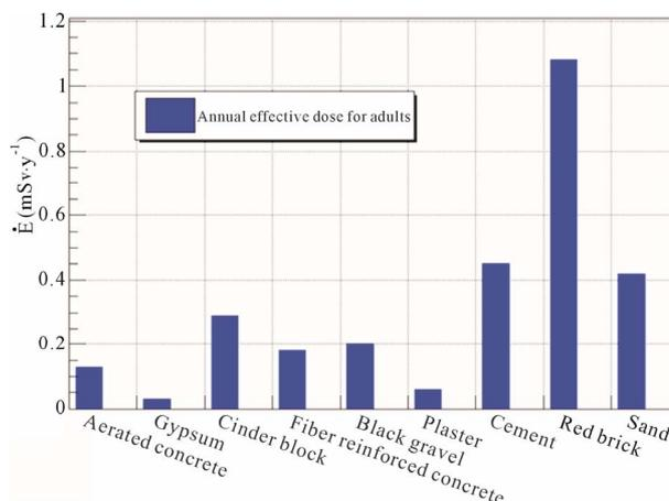
**Figure 4.** Annual effective dose  $\dot{E}$  from the tested construction materials.
