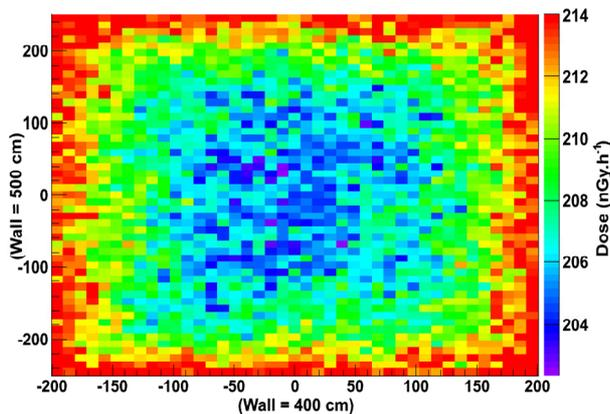
Figure 6. Absorbed dose distribution represented in 2D at 1 m height for a room built of red brick.
