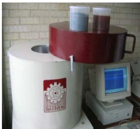
**Figure 1.** Low background scintillation detector and Marinelli containers.
