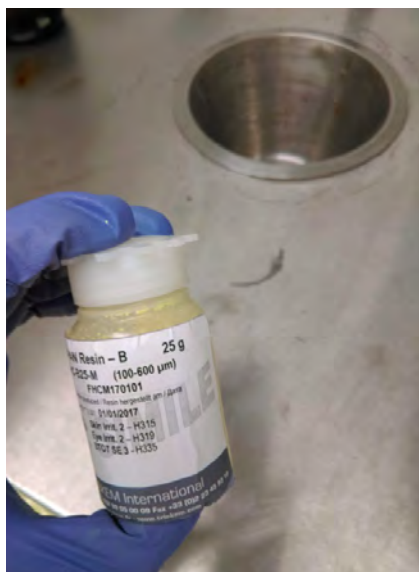
Figure 1. Triskem International AMP-PAN (ammonium molybdo phosphate embedded in polyacrylnitrile) resin cation exchanger.
