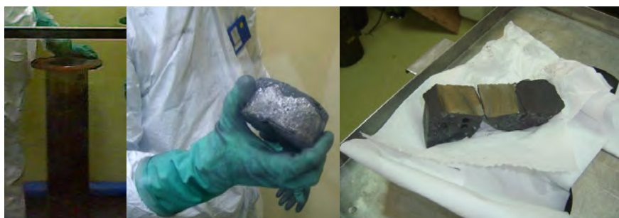
Figure 12. Uranium ingot obtained and cross-section of the sample.
