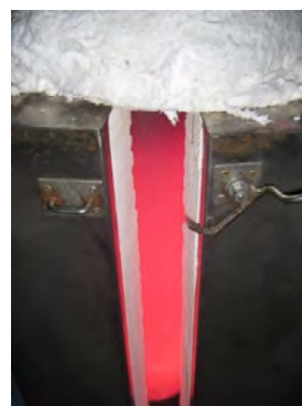
Figure 7. Magnesiothermy reactor, once the reduction reaction started.
