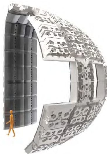
Figure 2. Blanket of the ITER. Source: ITER Organization. ITER Project web site.
