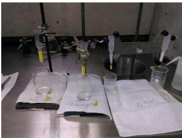
Figure 2. AMP-PAN filtration columns to trap ^{137}\text{Cs} from acid solution and exchange it into a basic solution.
