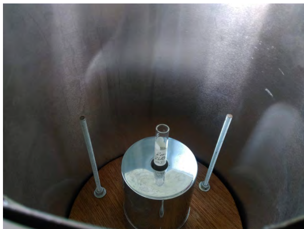
Figure 3. Activity detection of ^{137}\text{Cs} - ^{137\text{m}}\text{Ba} standard acid solution before filtration, and after recovery of radioactive pair in basic solution.
