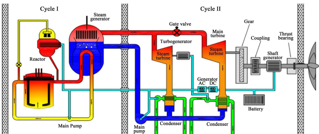
**Figure 4.** Simplified scheme of nuclear propulsion system in two-contour PWR cycle [15].
