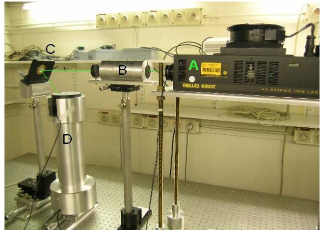
**Figure 1.** Layout of the OSL facility (A: Ar laser—B: Beam expander C: Mirror—D: tube with detector support, optics and PMT).
