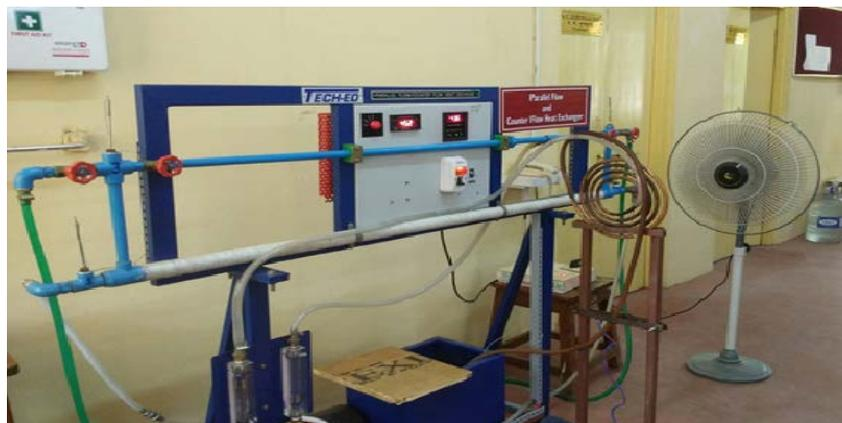
**Figure 1.** Experimental setup for spiral heat exchanger using Nanofluid as coolant.
