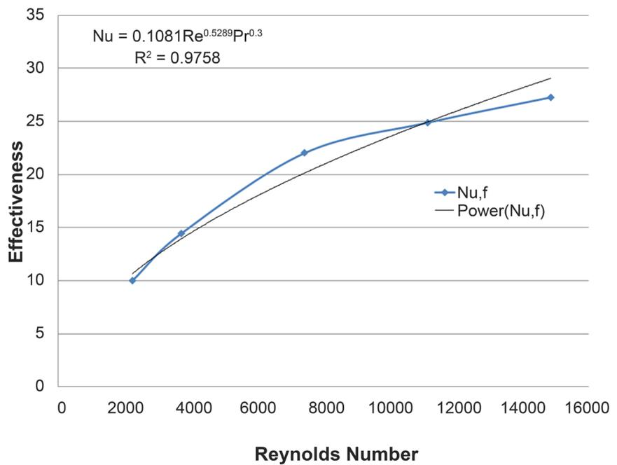
Figure 5. Nusselt Number vs Reynolds Number for 0.4% volume concentration of Nanofluid at 6.5 m/s air velocity.
