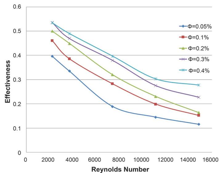
**Figure 7.** Effectiveness vs Reynolds Number at 5.5 m/s air velocity.
