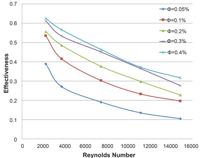
**Figure 8.** Effectiveness vs Reynolds Number at 6.5 m/s air velocity.
