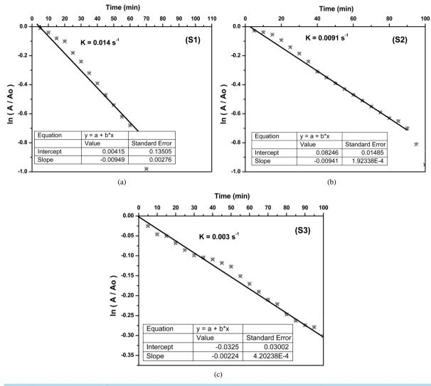
Figure 7. The kinetic curve of 4-NP reduction by AuNPs 4 nm in diameter in the presence of NaBH<sub>4</sub>.
