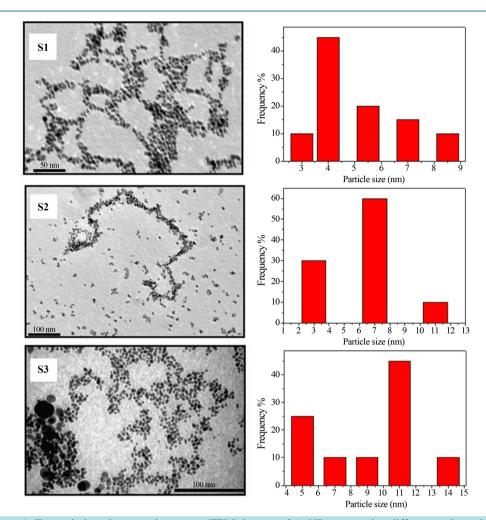
**Figure 1.** Transmission electron microscopy (TEM) images of AuNPs prepared at different molar ratios of chloroauric acid and trisodium citrate; sample S1 (20:7), S2 (20:20) and S3 (20:60). The average particle sizes estimated from images were 4, 7 and 11 nm for the samples S1, S2 and S3, respectively.
