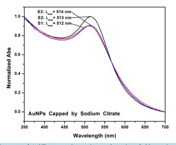
Figure 2. UV-VIS spectra of AuNPs prepared at various molar ratios of chloroauric acid and trisodium citrate; S1 (20:7), S2 (20:20) and S3 (20:60).
