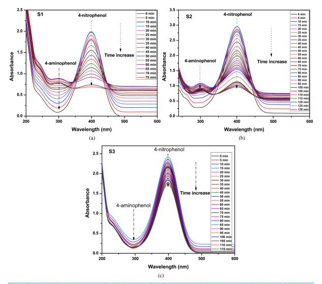
Figure 5. UV-VIS absorbance spectra for the reduction of 4-NP with NaBH<sub>4</sub> in the presence AuNPs with particle size 4 nm (S1), 7 nm (S2) and 11 nm (S3).
