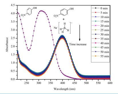
Figure 4. Measurements of the UV-VIS spectra of 4-NP over time with NaBH<sub>4</sub> at (400 nm) and without sodium borohydride at (317 nm).
