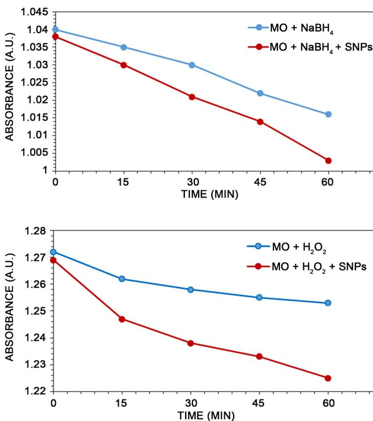
**Figure 3.** Degradation of the methyl orange solution ( $3 \times 10^{-4}$  M) in the absence and presence of SNPs (500  $\mu$ L) and 1 mL of NaBH<sub>4</sub> solution (0.001 M) or H<sub>2</sub>O<sub>2</sub> solution (0.001 M).
