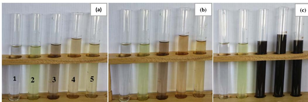
**Figure 1.** Photographs showing colour changes of silver nitrate solution (2 mM) after adding of extract of tangerine peel solution after reaction time: (a) 15 min; (b) 30 min; (c) 45 min. (1) silver nitrate solution (2) extraction of tangerine peel solution, (3) ratio of silver nitrate solution to tangerine peel solution 2:1, (4) 1:1, and (5) 1:2.
