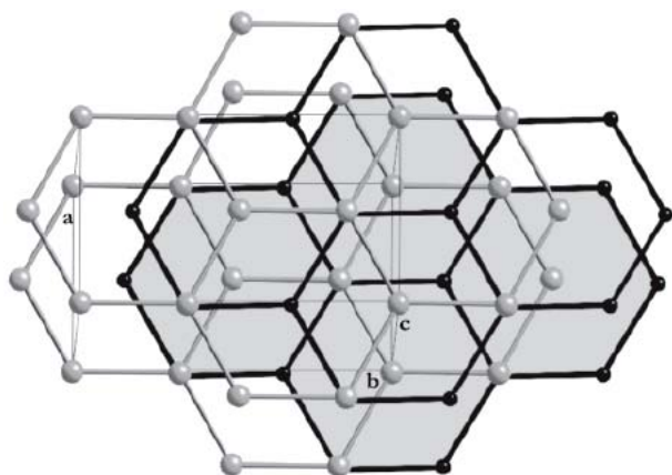
Figure 1. Stacking polytypism in kaolinite; Only the \text{Si}^{4+} ions (dark) and the \text{Al}^{3+} (light) are shown for simplicity. The view direction is perpendicular to the sheets and a shading has been added to the lower \text{Si}^{4+} layer. The thin lines denote the unit cell [14].
